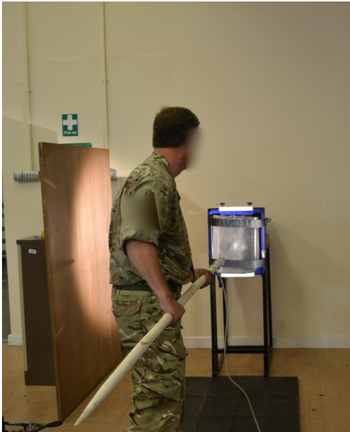
310 311 Figure 6: Participant performing spear thrusting in a block of PermaGel™. Hand position 312 was the most typical used by participants.
